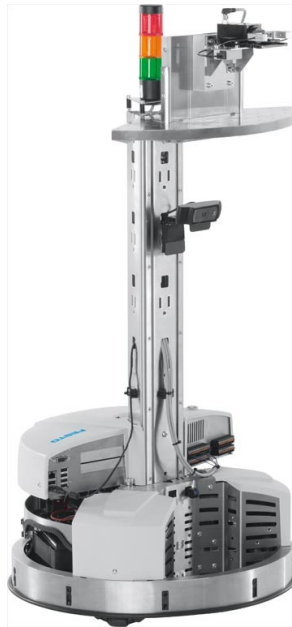
Figure G.1: Robotino shown with Tower, Segment Base, Gripper, and Signaling Lights
