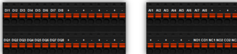
Figure 3.10: The I/O Interface of the Robotino Displaying the Connections
