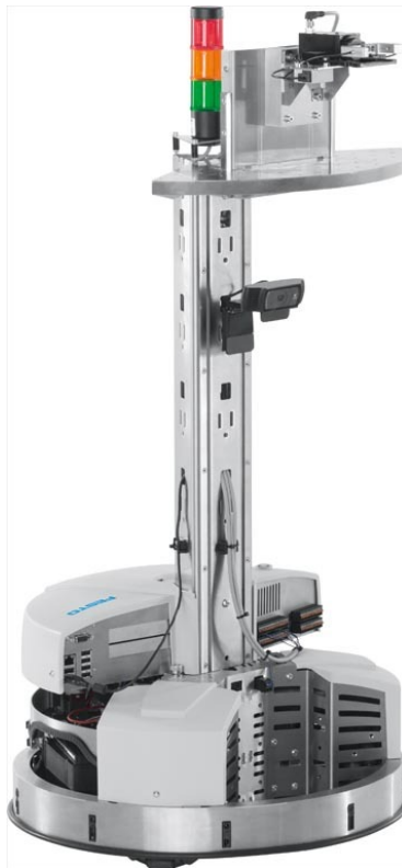
Figure 3.1: Robotino shown with Tower, Segment Base, Gripper, and Signaling Lights
