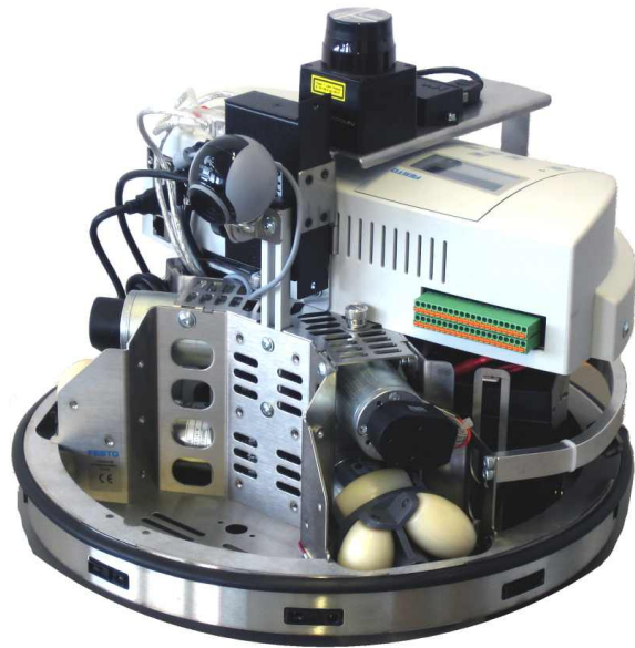
Figure 7.2: Showcasing Robotino with a Hokuyo Lidar Mounted
