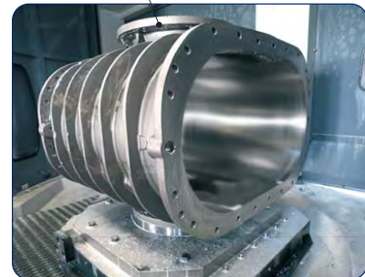
The precision milling and boring of the blower casing guarantee reduced tolerances and higher efficiency.
