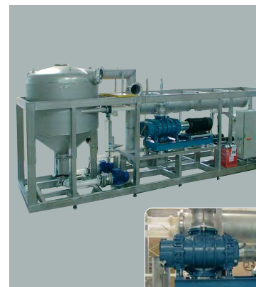
• Engineering: treatment of oil emulsions and cleaning liquids by means of thermocompression concentration system. Lobe blowers (RBS)
