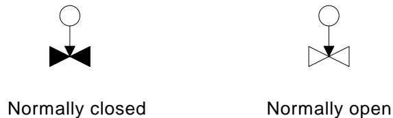
Figure B.35 - Valve normal position
