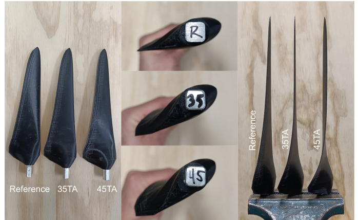
(b) Picture showing the different twist angle distributions.
