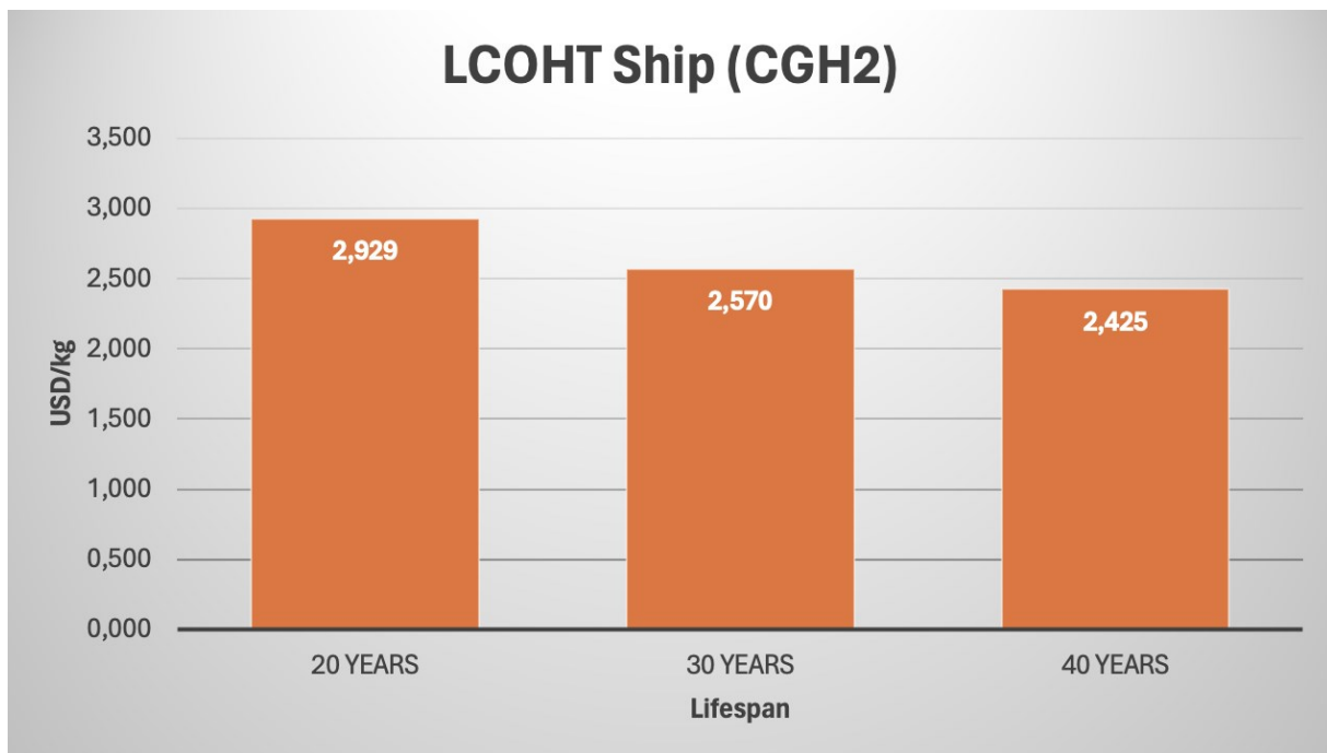
Figure 8: LCOHT for CGH 2 ships with lifespan of 20 years, 30 years and 40 years
