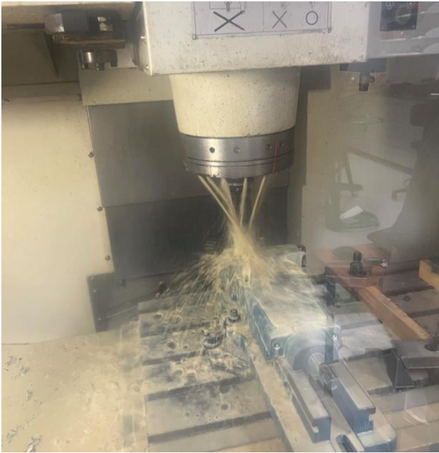
Figure 194 - CNC machining of bracket
