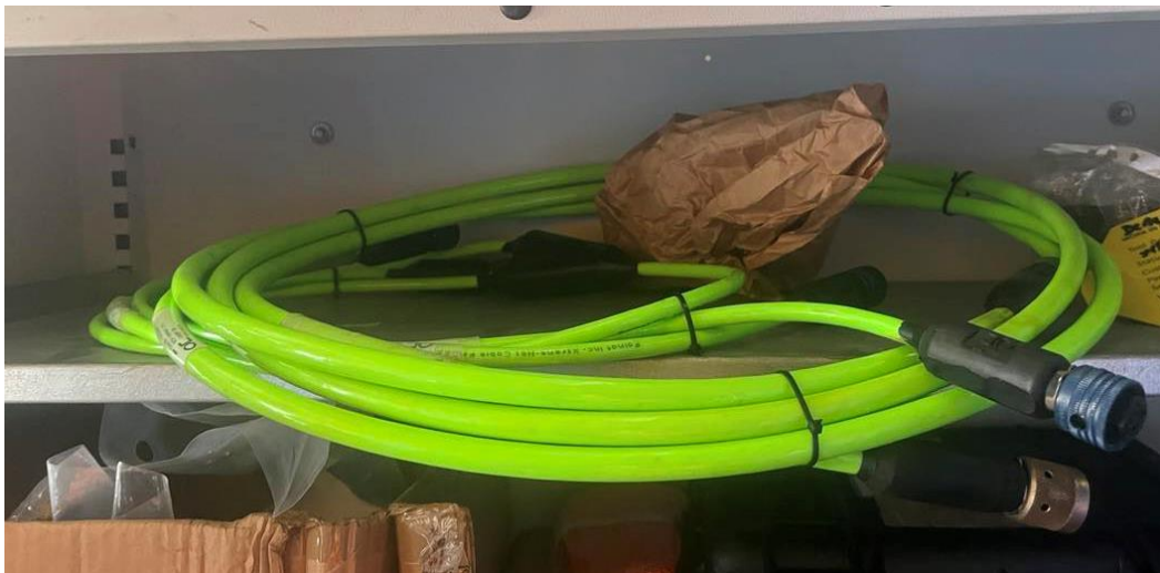
Figure 7 - Molded ROV cable with connectors (private photo)
