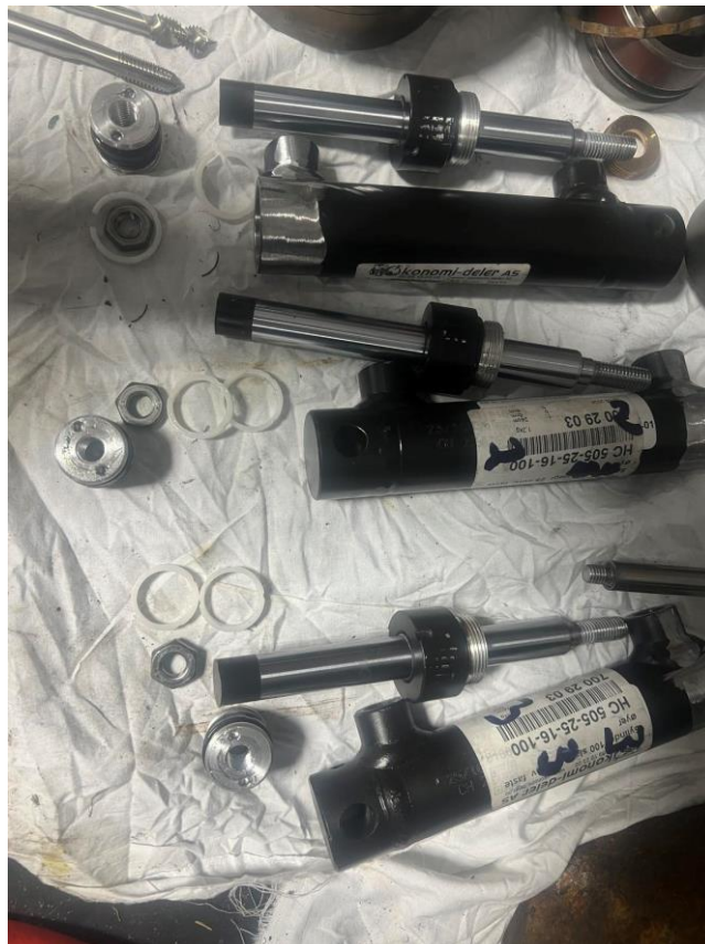
Figure 193 - Cylinders demounted for welding of flange
