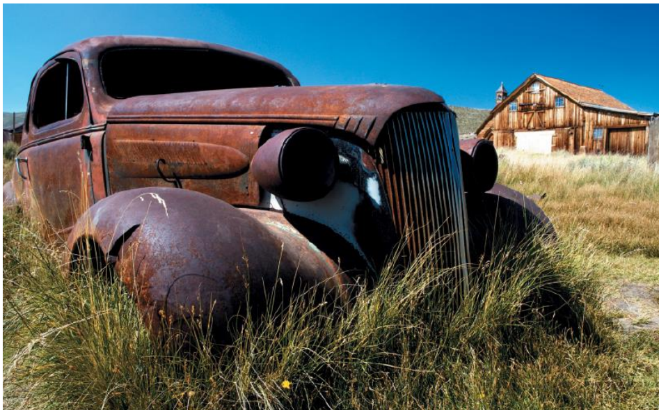
Figure 14 - Corrosion at the surface of a car with a plain carbon-steel body [24]
