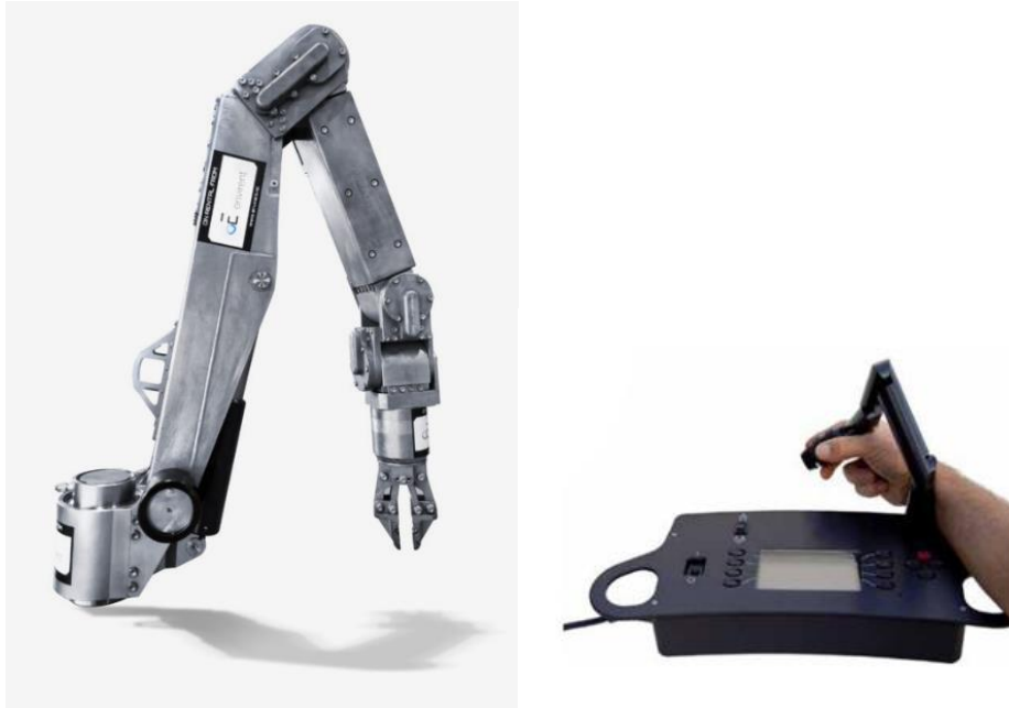
Figure 6 - Schilling T4 7-functions manipulator (left) [6], and controller (right) [7]
