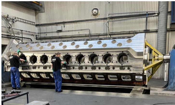
Figure 5 - Inside Bergen Engines' facility, two technicians surface treat one of Bergen Engines colossal engine blocks.
