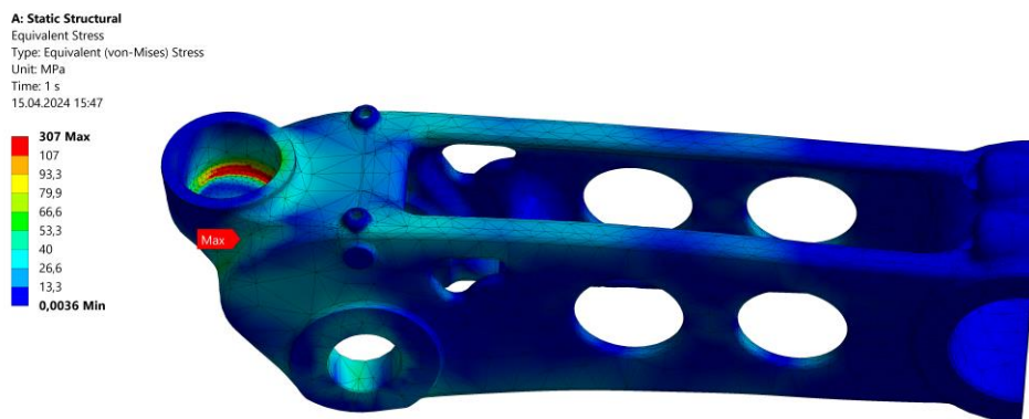
Figure 21 - Max Von Mises Stress [MPa] of the original swing arm.
