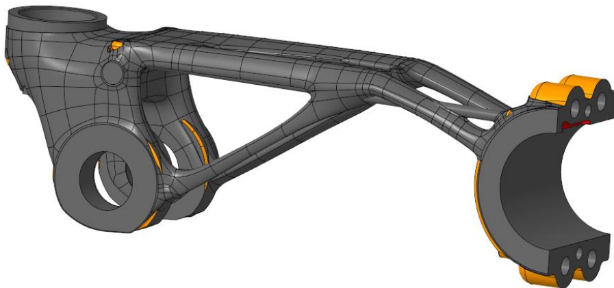
Figure 24 – Optimized design for the swing arm.
