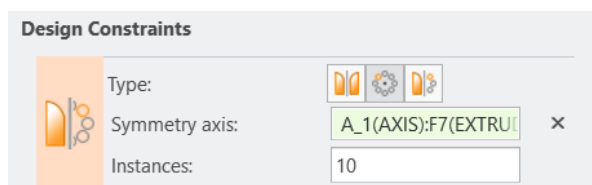
Figure 79 – Option for symmetry axis design criteria, Creo Generative.
