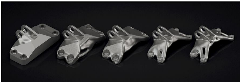
Figure 8 - Part optimized by Creo's generative design.
