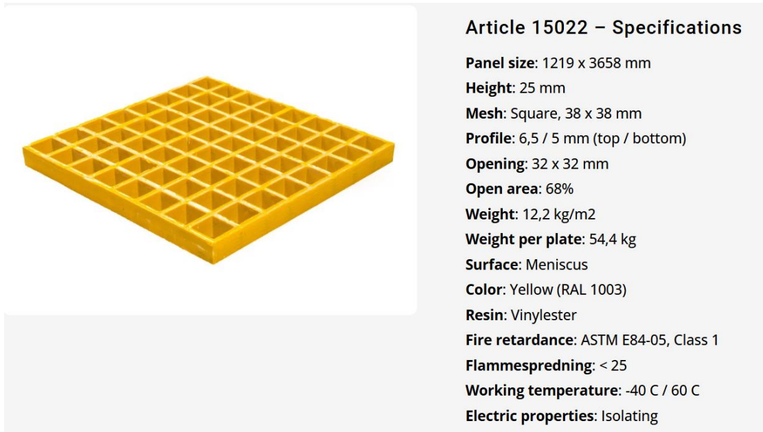
Supplementary Figure 5 - GRP grating specifications. [23]
