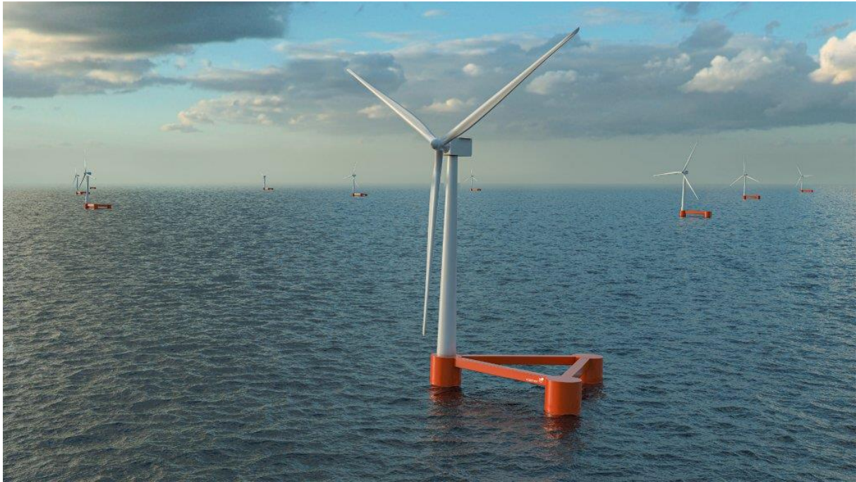
Figure 2-1. FOWT semi-submersible concept Equinor Scotland [45].
