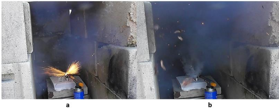
Figure 4.17 (a) Activation of TR with rapid sparks (b) explosion with flying debris and slight gas emission afterward. Also seen in Figure 4.3 b and c.
