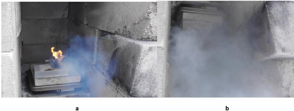
Figure 4.18 TR propagation on cell 2 initiates with flare and sparks (i) excessive whitish gas/smoke ejection from cell 2, extinguished flame. Also seen in Figure 4.8 i and j.
