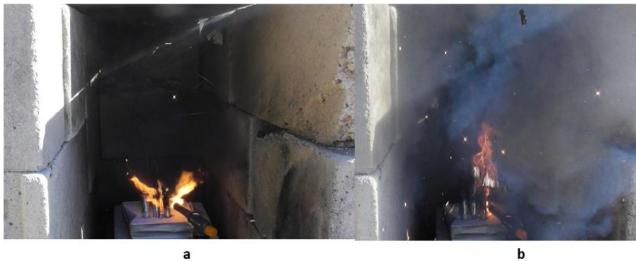
Figure 4.20 Li-ion 3x3 configuration 1cm spacing (experiment 2). (a) flare with sparks (b) explosion with flying debris accompanied by gas emission with radiation flame engulfed cell 1
