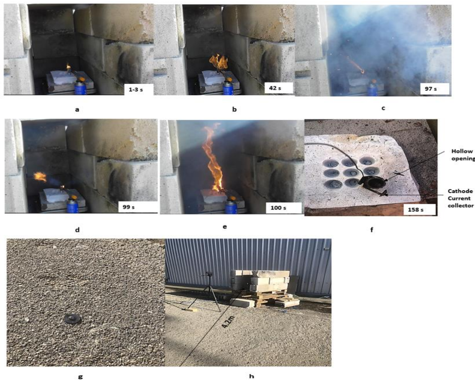
Figure B1 Initial external abuse process (b) safety vent activation with ignition of ejected gas (c) initiation of TR with rapid gas ejection with sparks (d) sparks with little gas ejection (e) ejection of flame touching the roof of the compartment (f) outcome of TR caused cell material displacement with the hollow opening on the cell and cathode current collector damaged (g) vent cover displaced (h) distance at which the vent cover was displaced from the experiment point.
