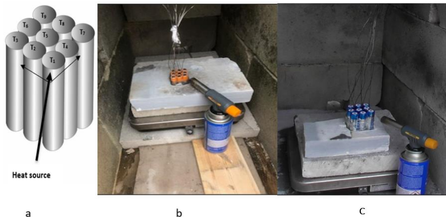
Figure 3.3 (a) shows the location of each thermocouple for both Alkaline and Li-ion cells and the direction of the Butane burner (b) shows the set-up of Alkaline 3x3 configuration, 0 cm spacing cells (c) shows the set-up of 3 x 3 configuration, 0 cm spacing cells.
