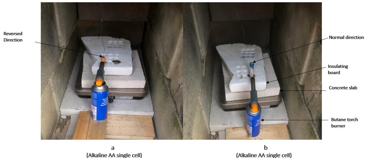
Figure 3.1 (a) shows the AA Alkaline cell placed in the hole in a reversed way with the anode exposed to the butane flame (b) shows the 18650 Li-ion placed in the hole in a normal way.
