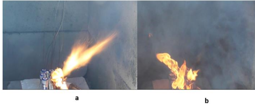
Figure 4.21 Li-ion 3x3 configuration 0.5 cm spacing (experiment 2). (a) initiation of TR with flare /sparks (b) Diffused flame engulfed cell with gas/smoke ejected during TR without explosion
