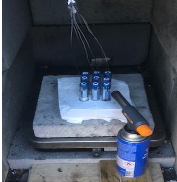
Figure 3.3 Li-ion 0.5 cm spacing apart with hole diameter in an insulating board.
