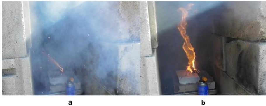
Figure 4.19 Li-ion single cell experiment 3. (a) Initiation of TR with flare/sparks with whitish gas emission (b) explosion accompanied by a flame jet touched the ceiling. See appendix.
