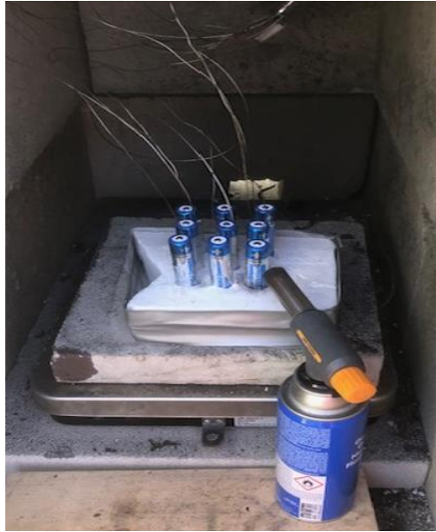
Figure 3.4 The photo shows one of the experiments with 3 x 3 configuration and 1 cm spacing.
