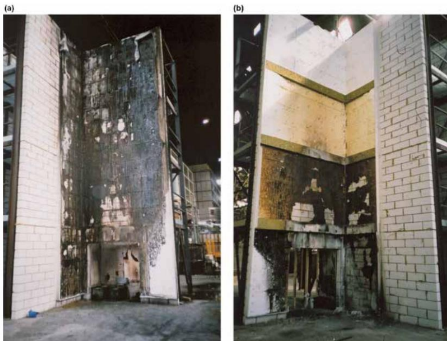
Figure 4 - (a) EPS system without fire barriers (b) EPS system with Fire Barriers - Source: BR135:2013
