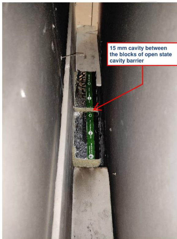
Figure 24 –The OSCB blocks installed within the experimental setup with a gap in between.
