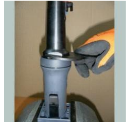
Using the spanner provided, unscrew the pneumatic cutter in a clockwise direction
