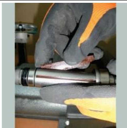
Put the blades back in, with the tapered side on the inside.
