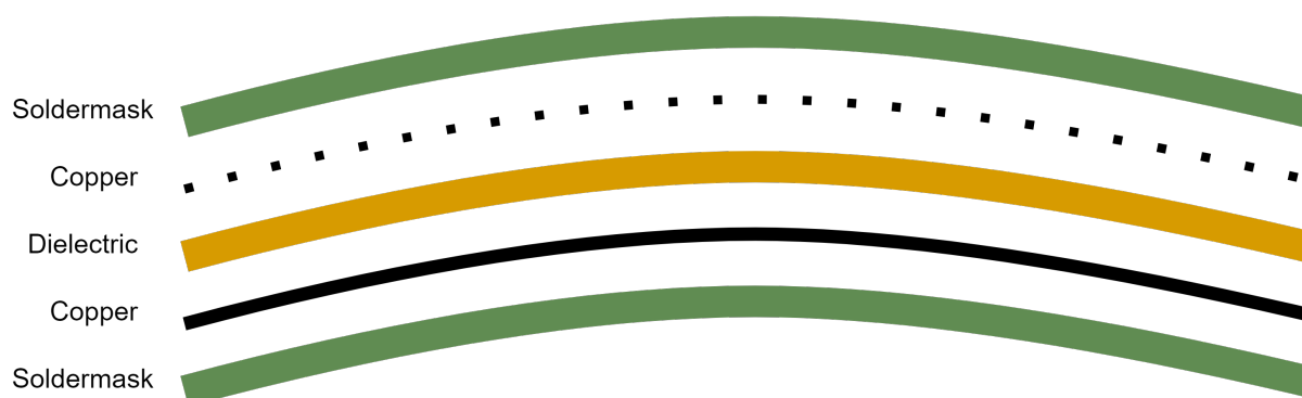
Figure 4.28: Warping as a result of copper imbalance
