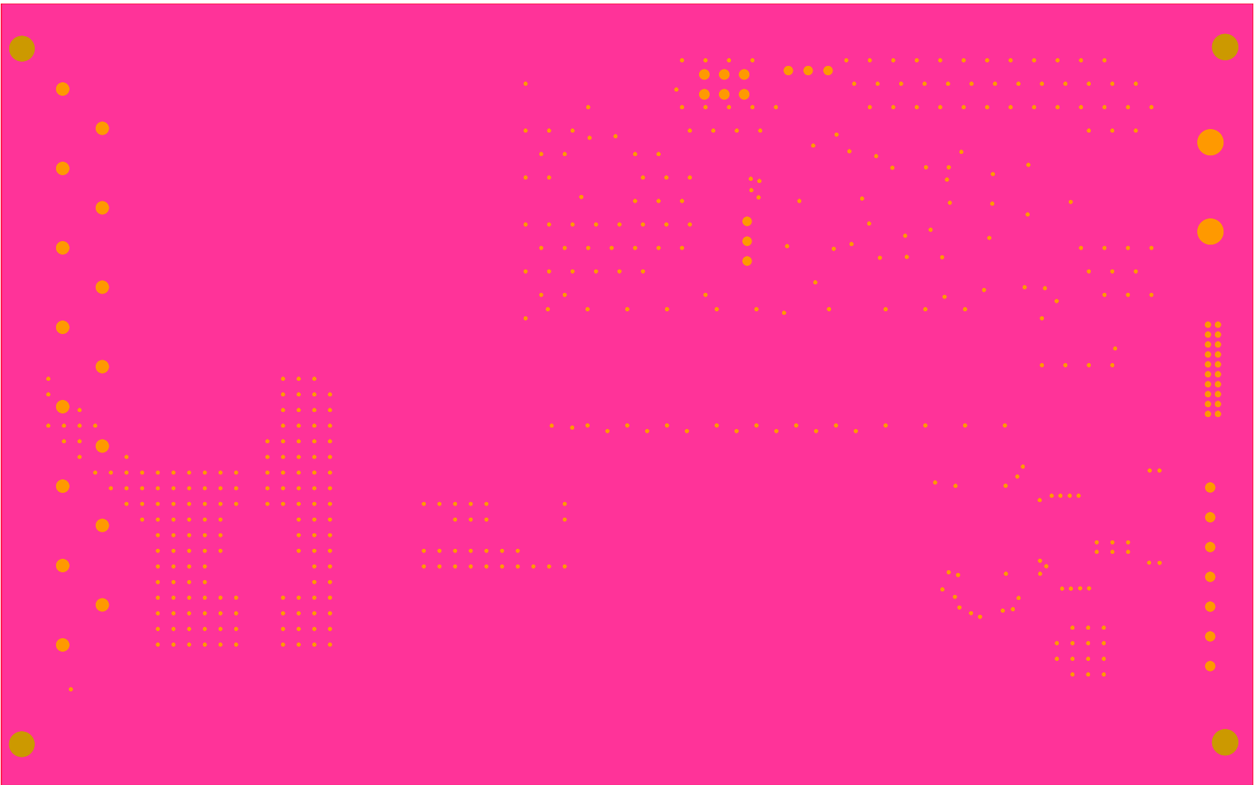
Figure D.3: Monitor Board layer 2 - Shield 1
