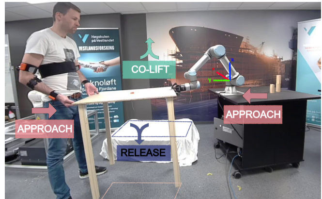
Fig. 1: Frame-capture from co-lift experiments using IMUs for human motion estimation and an EMG-sensor to open/close the gripper. The co-lift states of APPROACH, CO-LIFT and RELEASE, and the pick and place locations, are illustrated.
