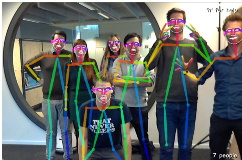
Fig. 2.4: A sample of the multiple human pose estimation using OpenPose Source:[89]
