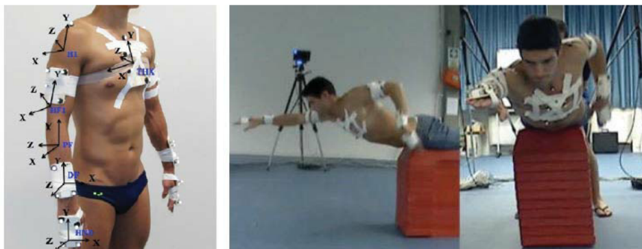
Fig. 2.6: An example use case of IMUs in swimming motion recording Source: [110]
