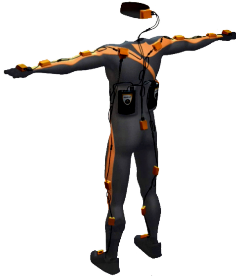
Fig. 1.5: MVN system which consist of 17 IMUs by the Xsens company Source: [19]
