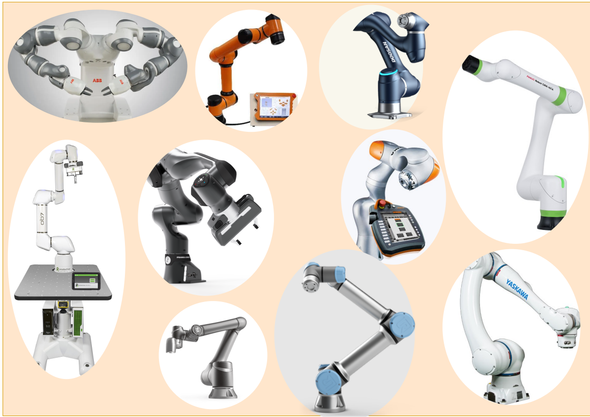
Fig. 1.3: Common cobots in the market today. From top left to bottom right: ABB YUMI , AUBO i5 , Doosan A0509 , FANUC CRX , Productive Robotics OB7 , Franka Production 3 , KUKA LBR iiwa , Techman Robot TM14 , Universal Robots UR5e , Yaskawa HC20DTP
