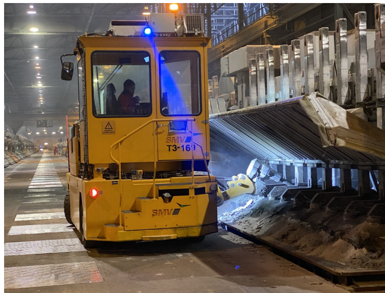
Figure 5.2.1: A crust breaker chiselling out a butt.
