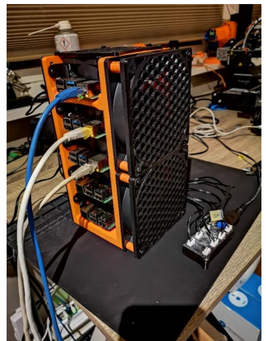
Figure 27 The final build of our raspberry pi cluster
