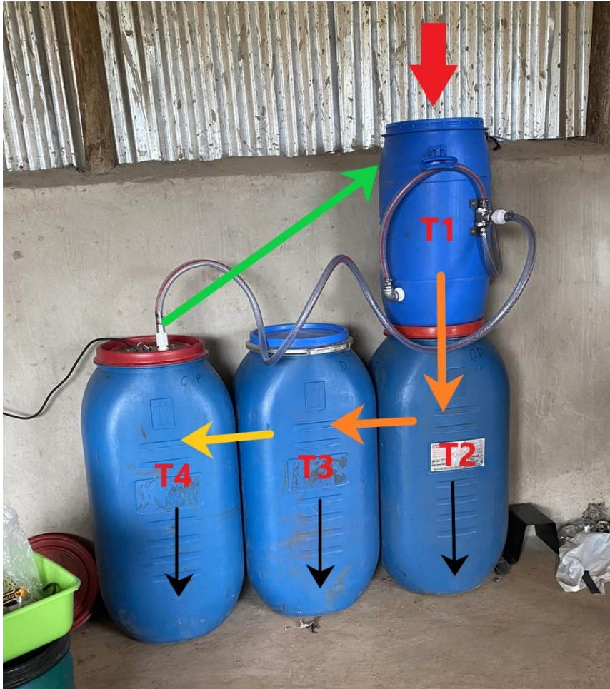
Picture 17 - Washing System Flow Chart (Langseth, 2023)
