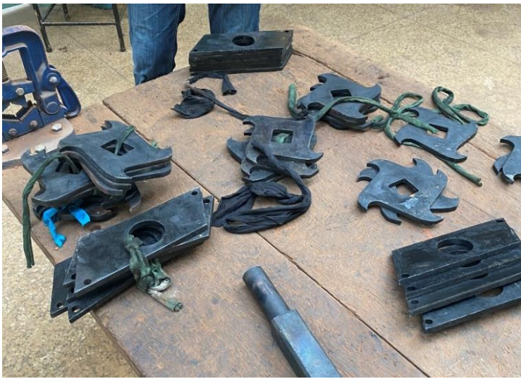
Picture 8 - Illustration of coating on all shredder parts (Langseth, 2023)
