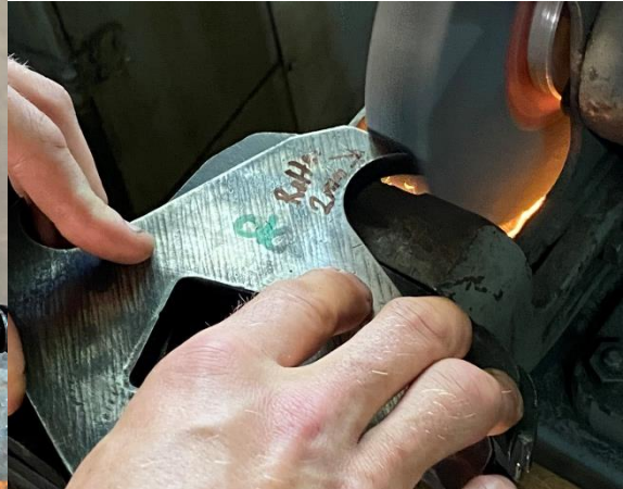
Picture 14 – Grinding rotating blades (Langseth, 2023)
