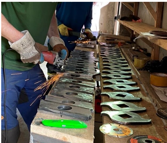
Picture 15 – Grinding Stationary Blades (Langseth, 2023)
