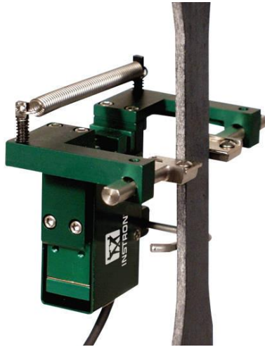
Figur 12 - Tverraksial "clip-on" ekstensometer. [10].
