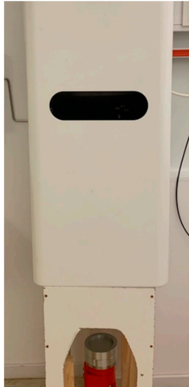
Figure 2. The closed hand dryer machine used in the study. The Oxoid Air Sampler is placed at air outlet from the device.
