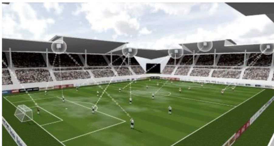
Figure 1. Principles of tracking by the ZXY system. Transponders worn by the players respond to signals sent out from beacons at known positions around the pitch. The players' positions are calculated from the recorded replies. Photo taken from the ZXY brochure, also available at https://www.nacinc.jp/analysis/sports-tracking/zxy-arena/ , accessed on 10 March 2023.
