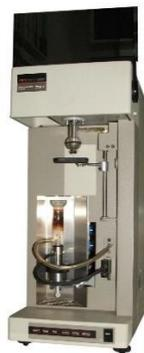
*Figure 22 – Example of a thermogravimetric analyser [70]*
