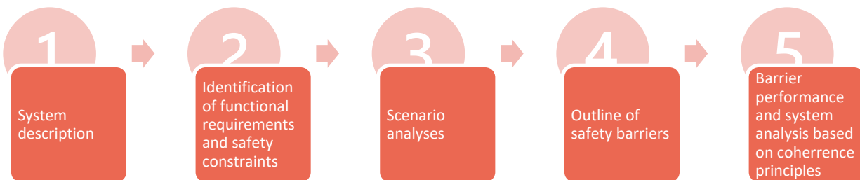
Figure 25 STS fire safety engineering framework [44]
