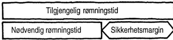
Figure 81 Illustration of ASET, RSET, and safety margin in the 1997-2007 guides to TEK [33, 52, 53, 54]
