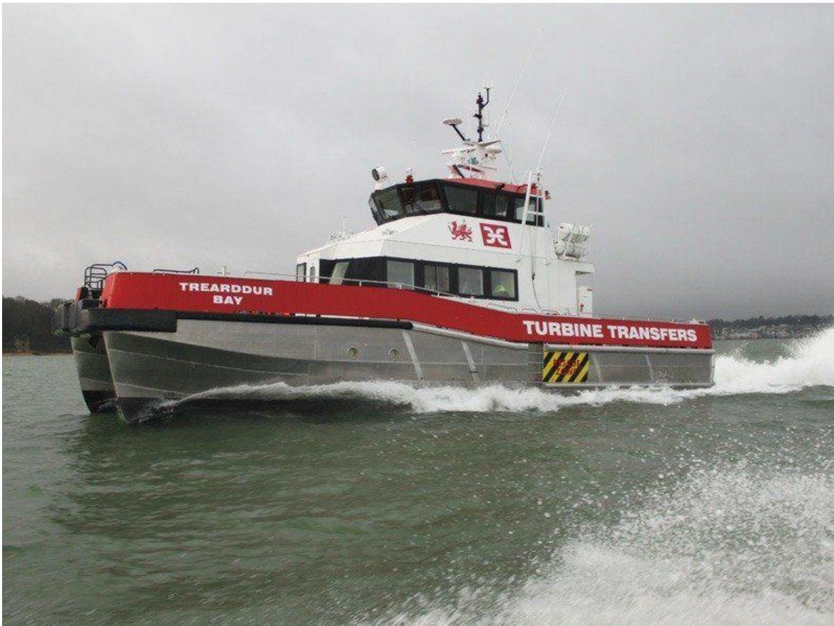
Figure 30 - Wind turbine transfer vessel. (Aluminium Marine Consultants, 2019-2022).
