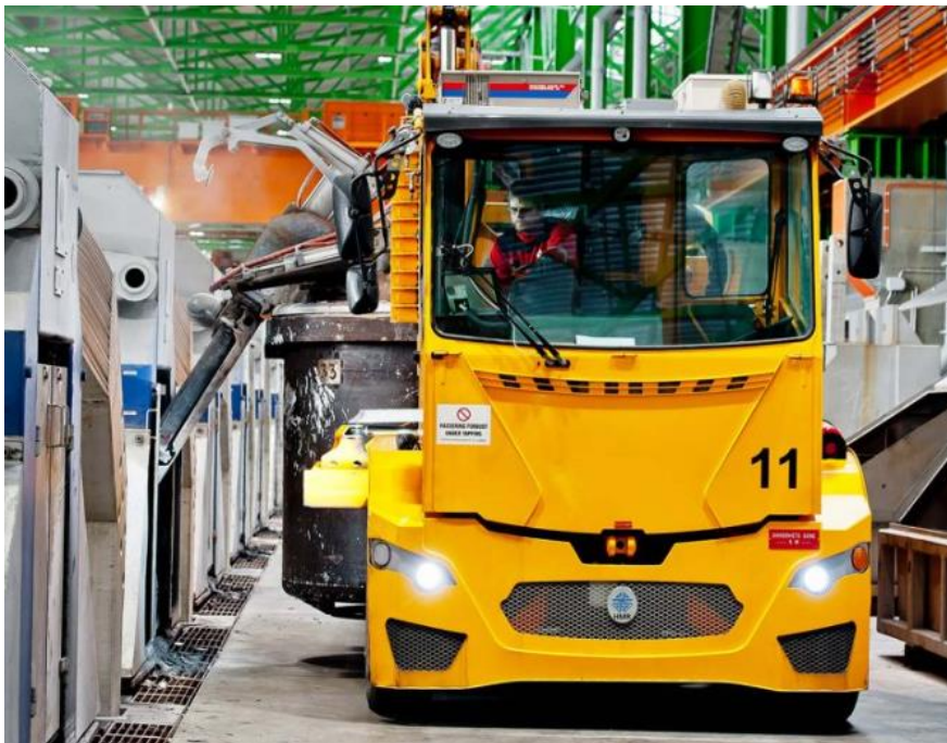
Figure 10 - A specialized vehicle for transporting liquid aluminum. (Aluminium INSIDER, 2023)
