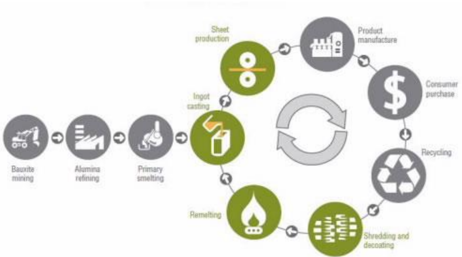
Figure 36 - Aluminium life cycle, including steps for recycling. (Husband, 2012).
