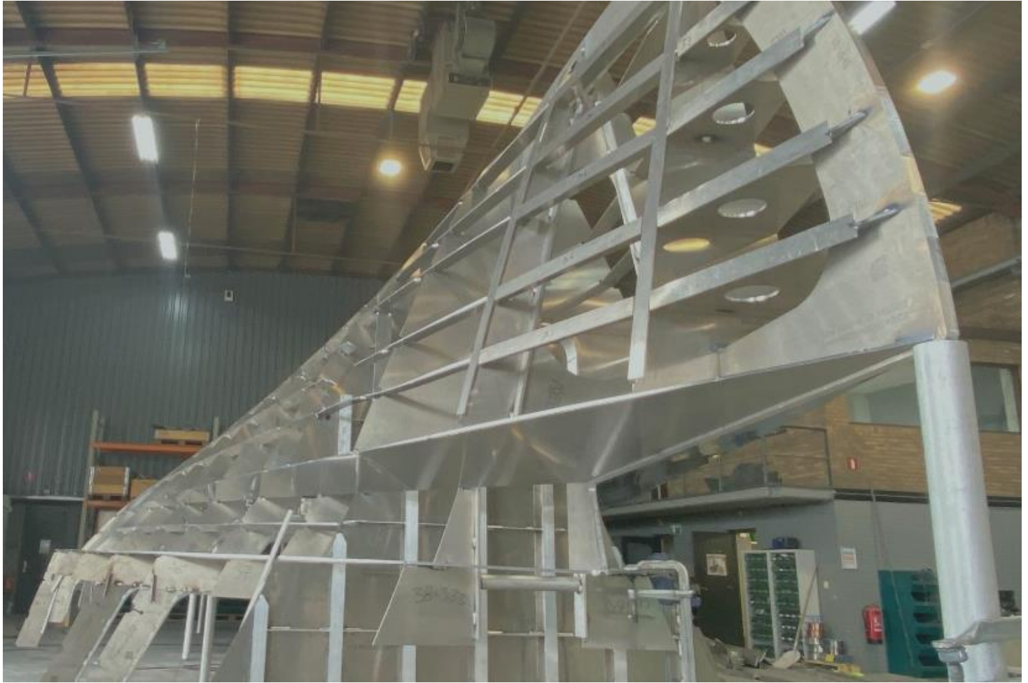
Figure 17 - Construction of a ship's hull with 5083 alloy. (Speira, 2022).
