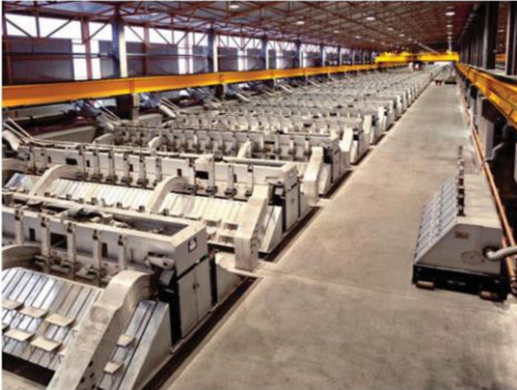
Figure 8 - Aluminium electrolysis potroom. (Kvande, 2014)
