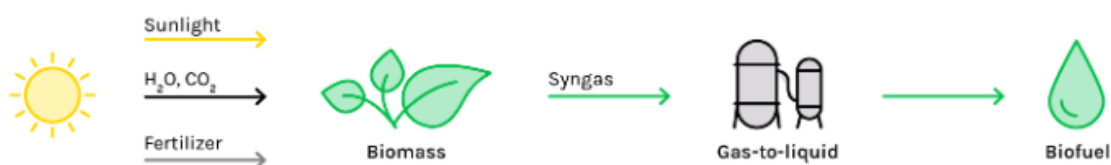
Figur 2-5. Prosessen for å fremstille biobrennstoff. ( https://synhelion.com/news/synthetic-fuels-explained ).
