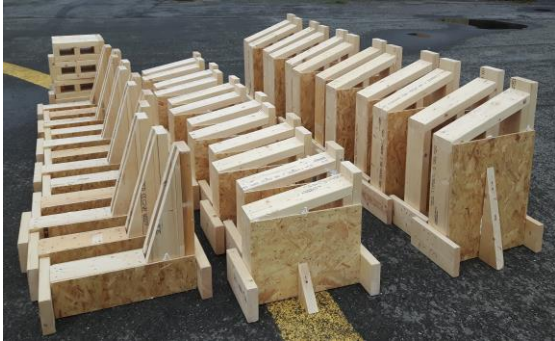
c. Support legs for heeling the Tromsø corridor at 10° and 20° of heel.
