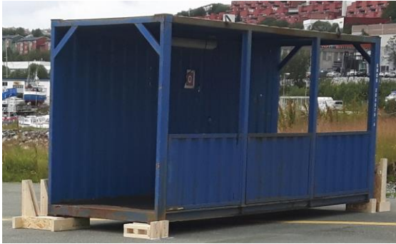
a. A steel corridor section used in the construction of the Tromsø corridor at 0° of heel.
