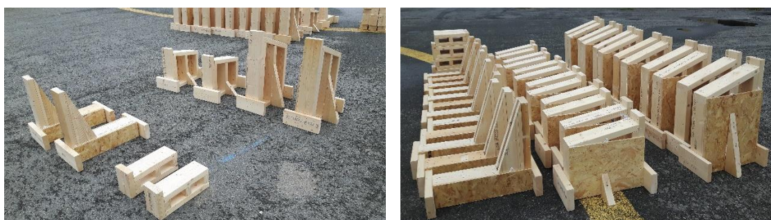
Figure 12: The container legs for 0^\circ , 10^\circ and 20^\circ in Arcos safety centre (Azizpour et al., 2022b)
