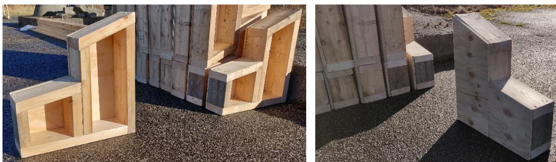
Figure 17: Corridor legs for heeling the corridor to 10^\circ and 20^\circ (Azizpour et al., 2022b)
