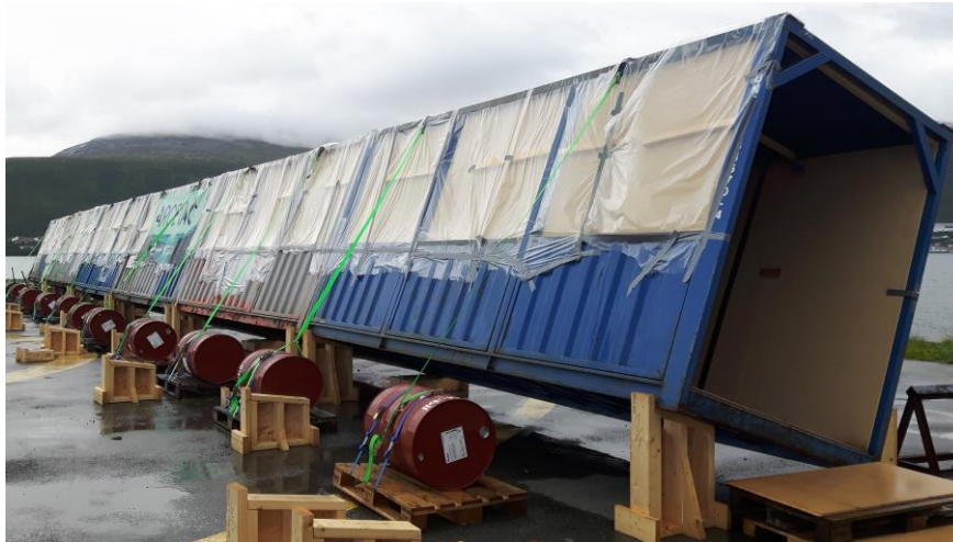
S2: The Tromsø test facility heeled at 20°
