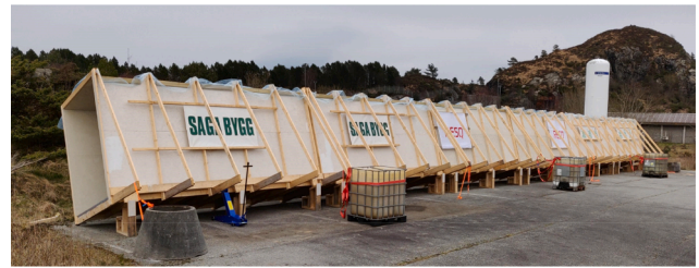
Fig. 2. The Haugesund test facility heeled at 20°.
