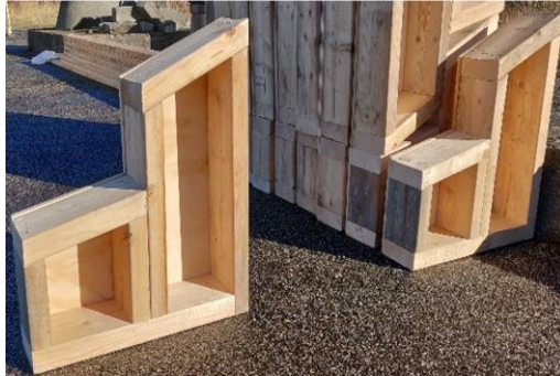
d. Support legs for heeling the Haugesund corridor at 10° and 20° of heel.
