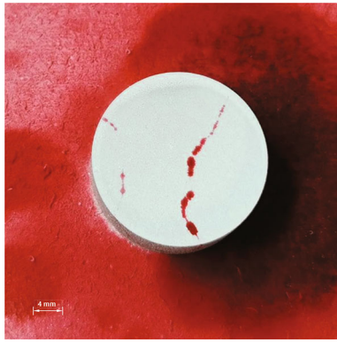
Fig. 8—Specimen with applied dye penetration test.
