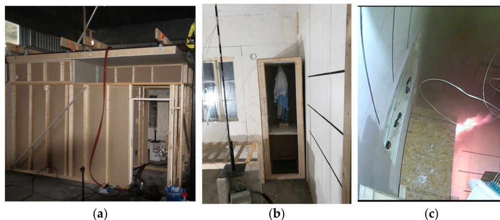
Figure 2. (a) The façade of the apartment; (b) fire load in the closet; (c) 115 s after ignition.
