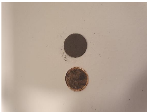
Figure 28. Failed anode (21 st March).
