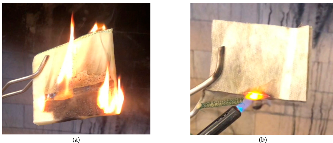
Figure 6. Initial Ignition Tests: (a) Flaming combustion of filter test specimen; (b) ignition test demonstrating glowing glass fibers.
