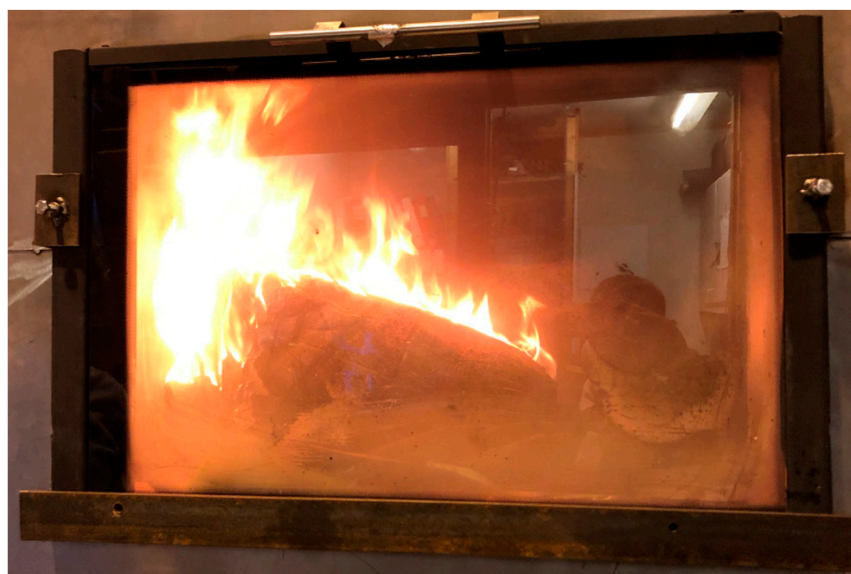
Figure 13. Used filter bag cassette tested at 200 °C. Photo taken 4–5 s after a rapid transition to flaming combustion.
