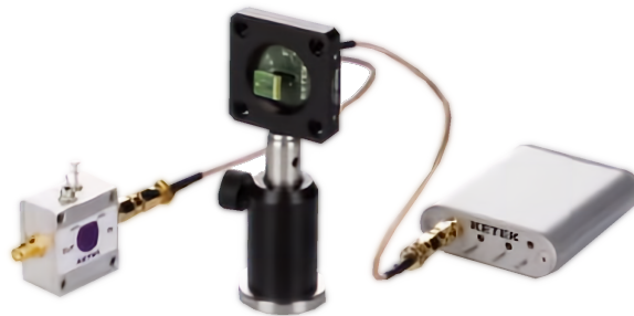
Figure 1.3: The Ketek Silicon photomultiplier evaluation kit. © Ketek
