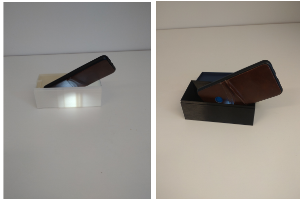
Figure 4.2: Light-tightness test of white and black PLA respectively.
