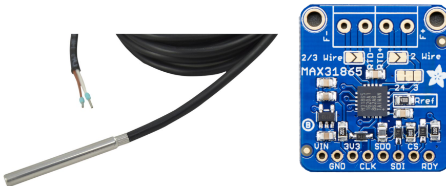
Figure 2.5: A PT1000 sensor and a MAX31865 breakout board. © Adafruit
