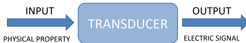
Figure 2.6 – Transducer input and output signal
