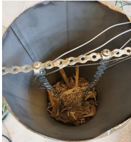
Figure 3-5 - Steel construction used to keep thermocouples at the same location.
