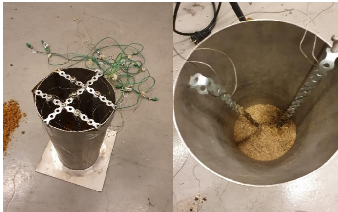
Figure 3-1 – Left: Overview of experimental setup in the preliminary experiments. Right: The expansion of the pellets.
