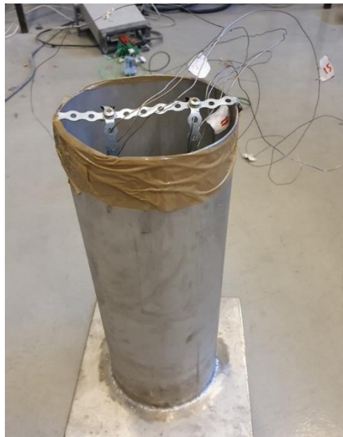
Figure 3-4 - Steel tube used in experiments. The metal-band construction is used to keep the thermoelements in place.
