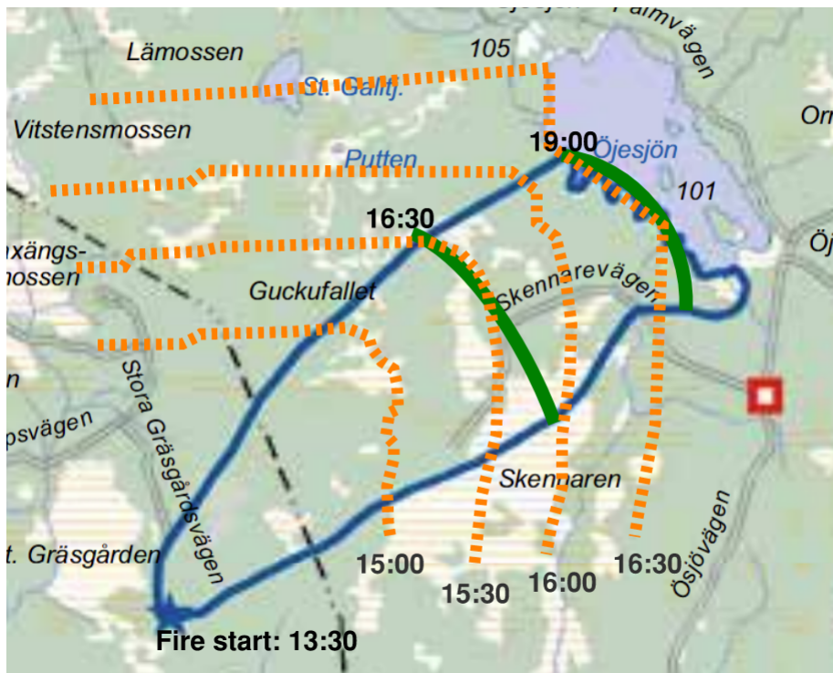
Figure 4.3.2-1: Comparison between the simulated fire and the reported timeline. Green lines illustrates the reported fire spread and orange lines the simulated fire spread.
