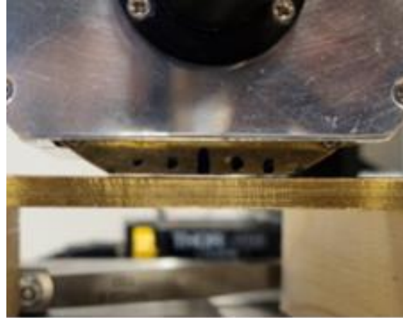
Figure 3.8 Close-up FKP and brass sample; starting point for experiment 50 \mu\text{m} initial distance
