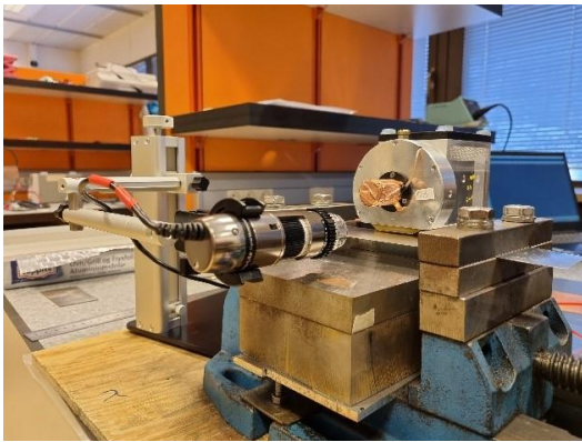
Figure 3.2 Test set-up with vice, FKP and camera microscope
