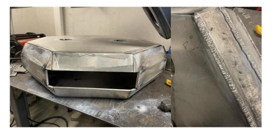
Figure 30 - Floater Unfinished (Left) and Weld Beads (Right)
