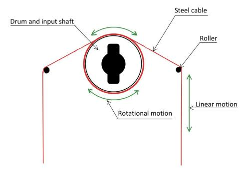
Figure 46 - Illustration of steel cable placement
