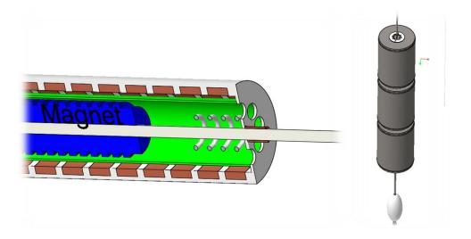
Figure 18 - Linear Generator with components (Left) and Linear Generator (Right)
