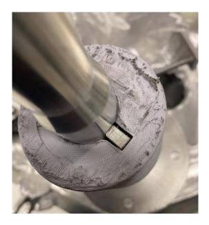
Figure 47 - Drum with keys inserted
