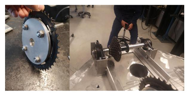
Figure 37 - Sprocket Flange Assembled (Left) & Output-shaft assembled (Right)
