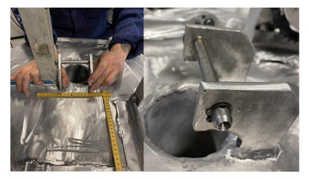
Figure 43 - Installing Rollers (Left) and Finished Rollers (Right)
