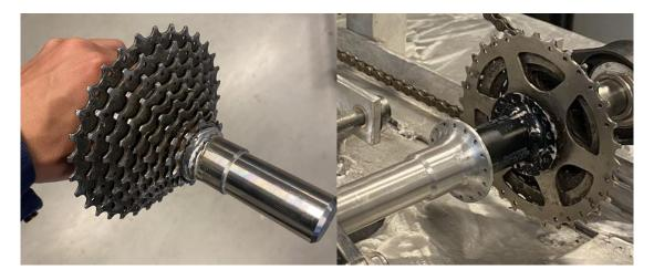
Figure 39 - Steel shaft welded to gears (Left) & Aluminium shaft welded to flange (Right)
