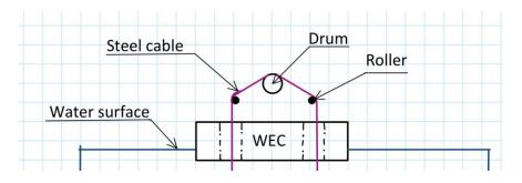
Figure 41 - Illustration of roller
