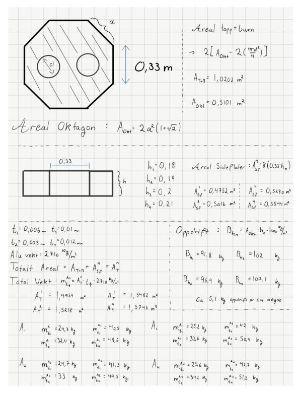
Figure 22 - Buoyancy Calculations
