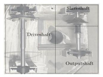
Figure 34 - Illustration of the different shafts
