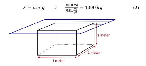
Figure 3 - Submerged Vessel
