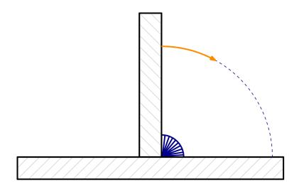
Figure 28 - Illustration of motion in the material due to welding
