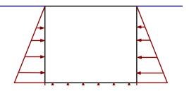
Figure 2 - Hydrostatic Pressure on Submerged Vessel
