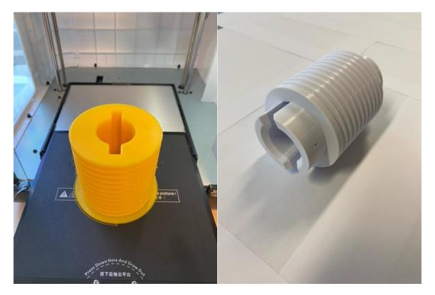
Figure 35 - First 3D print (Left) and Final Redesigned Drum (Right)
