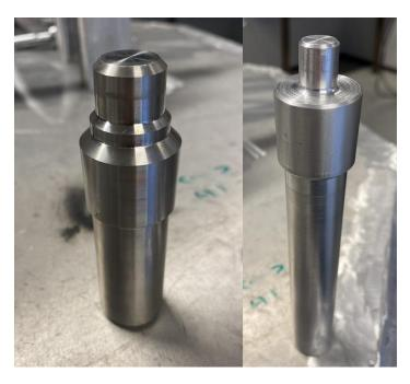
Figure 38 - Steel Axle (Left) and Aluminium Axle (Right)
