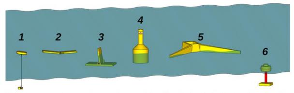
Wave energy generators come in many shapes and sizes. Some designs bob or float on the surface (1, 2, 4) or flip from side to side (3). Another type harnesses energy from waves as they crash onto shore (5). Still others sit near the sea bottom (6).
