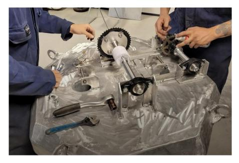
Figure 23 - Lubricating gear with Silicone-penetrant
