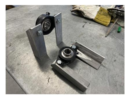
Figure 33 - Bearings mounted on L-50x6 Profiles
