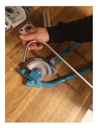
Figure 44 - Bending of steel rod
