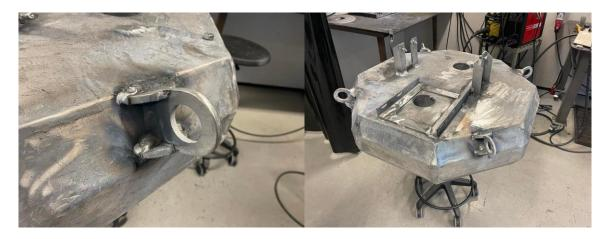
Figure 45 - Mooring attachment (Left) & Placement of Mooring attachment points (Right)
