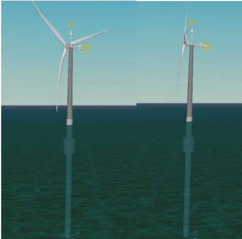
Figure 33: Turbine before and after yawing[38]
