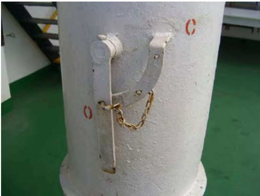
Figure 2.11: Clear marking of “Close-Open”
