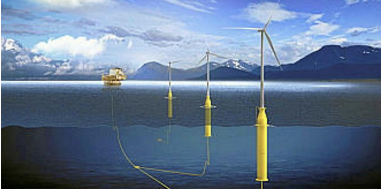
Fig. 8 Illustration of the Hywind Tampen array with the spar buoy foundation, source Equinor
