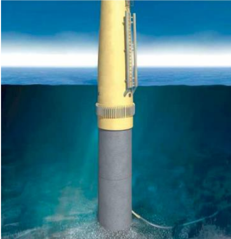
Fig. 9 Monopile foundation, from [26]
