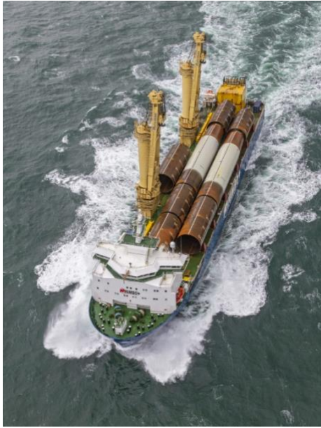
Fig. 24 HLV transporting monopoles, from [58]
