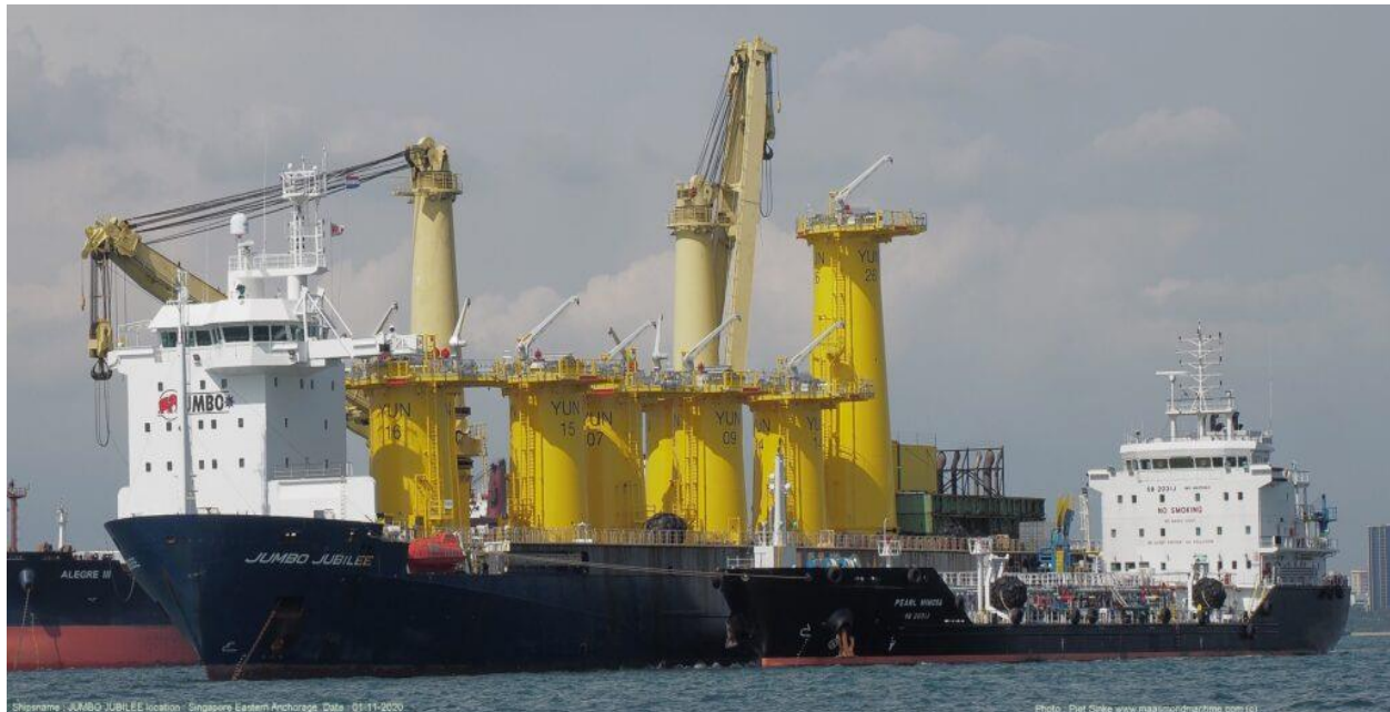
Fig. 23 Transition pieces transported on an HLV, from [58]
