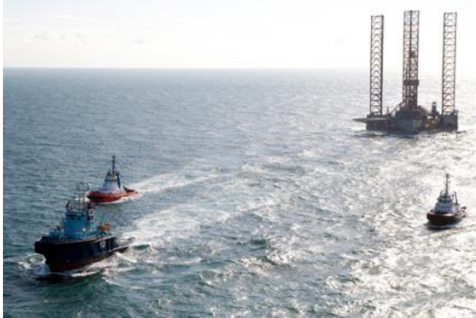
Fig. 21 Jack up barge towed to operation site, from [55]
