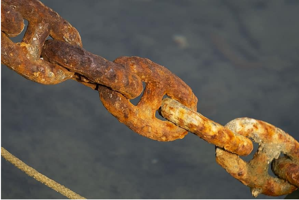
Figure 6 - Corrosion on chain
