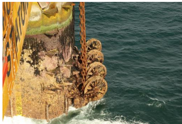
Figure 5 - Example of fairlead [18]
