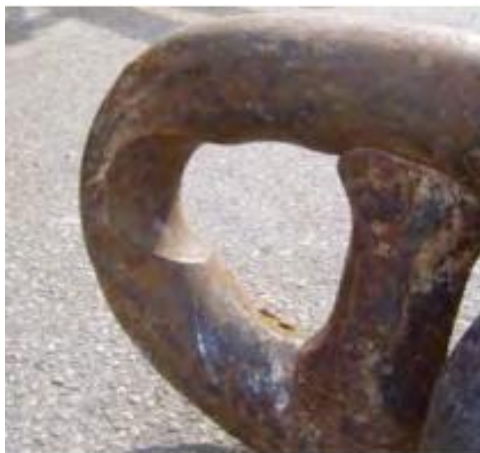
Figure 8 - Adhesive wear in the interlink zone
