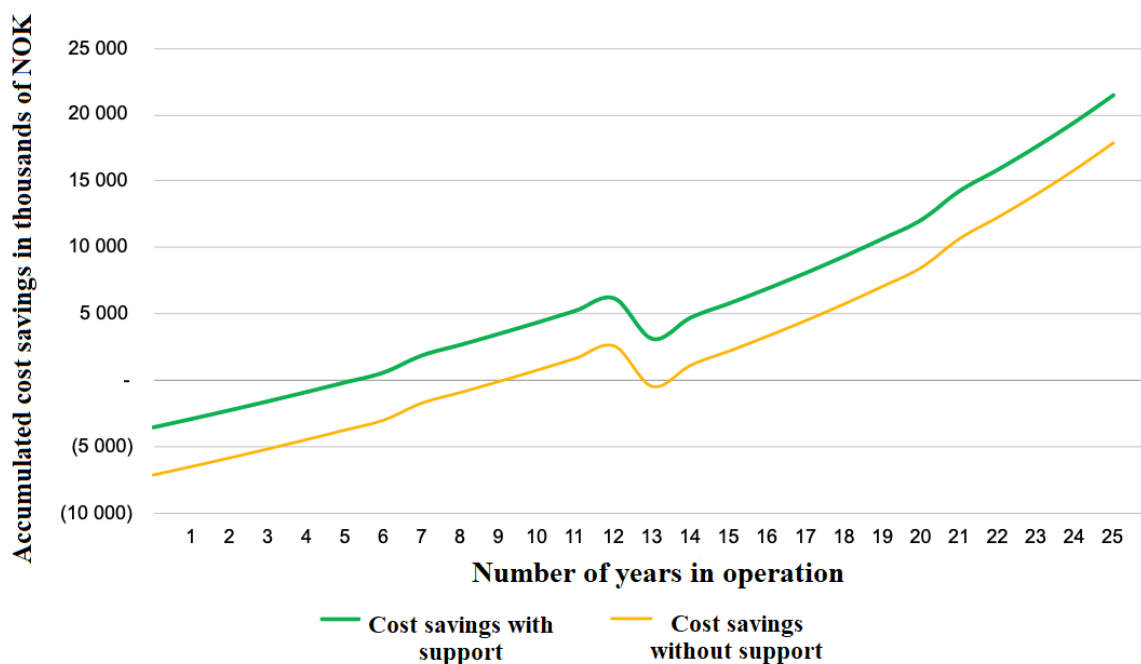
Figure 10: Cost savings with and without support for Boat 1, scenario 2 in the south of Norway
