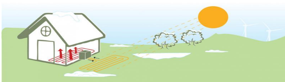
Figur 14 Jordvarmepumpe (NOVAP, u.å.)
