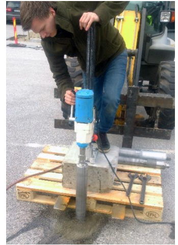
Figure 11: Drilling hole for sensor
