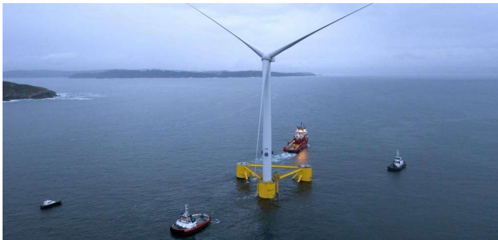
Figure A.6 Tow-out of the type Wind Float, 2019, from [A.8].
