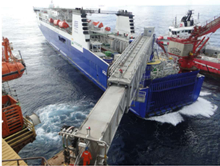
Figure 3.1 Uptime Gangway installed on a vessel (Illustration)
