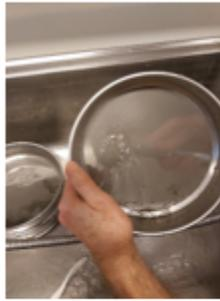
Picture 4: Concentrating the material in the sieve. Make sure that no material is left in the sieve after transferring it into the beaker.
