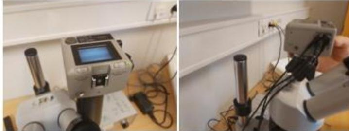
Picture 2: a) Camera mounted on the stereomicroscope. b) Position of the different cables when the system is connected.
