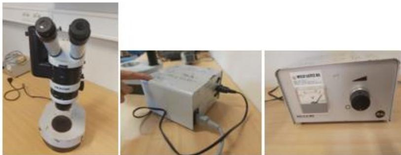
Picture 1: a) Stereomicroscope. b) Power supply with position of cables when the system is connected. c) 12 (15) V power supply.
