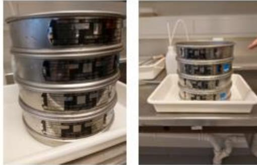
Picture 2: a) The set-up of the sieves, mesh sizes (from the top): 2 mm, 250  $\mu\text{m}$ , 125  $\mu\text{m}$  and 63  $\mu\text{m}$ , b) sieves are placed in a plastic tray in case of spilling of the samples.
