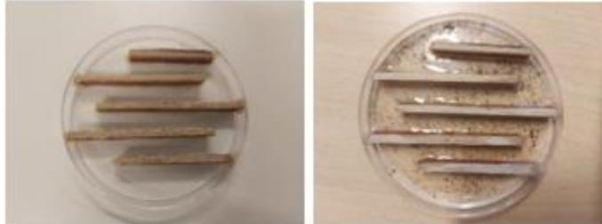
Picture 4: Counting chamber. Each line is suited to the 12X magnification. a) Empty and cleaned. b) Holding a subsample. This density of the particles in this sample is easy to investigate, but one may use a somewhat higher density of particles
