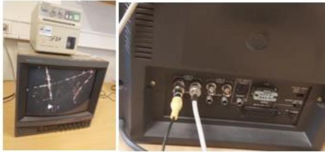
Picture 3: a) Monitor/video and video printer. b) Position of different cables (video in, video out) in monitor when the system is connected.
