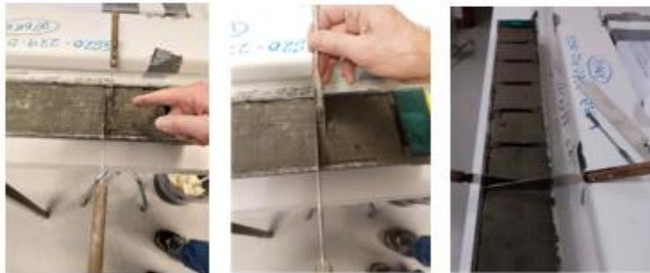
Picture 1: a) Two spatula defining the sampling area, b) sediment sampling, using a mini-spatula, c) sampled sediment core.
