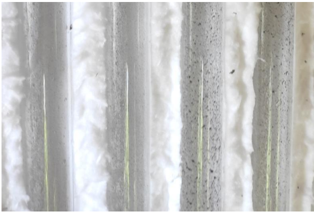
Figure 11: Local contamination of glass tubes by nanofluids with MWCNT concentration > 0.01\% wt.
