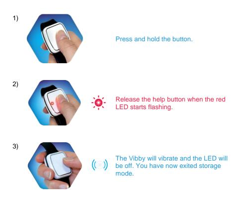
After exiting Storage Mode, the Vibby will automatically enter Demo Mode for 5 minutes before entering Active Mode (e.g. ready for use).
