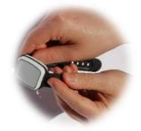
Holding onto the existing wrist strap and the Vibby gently pull until the retention features click out of place. Repeat this process for the remaining side of the strap.
