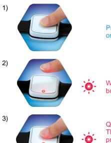
Press the button until the red LED turns on.
