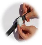
Pull the top of the wrist strap onto the Vibby. Ensuring the retention features line up with their holes and the edges fall within the enclosure.
