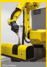
• *i*RTorchMate Prevents alignment issues by keeping the tool centre point exactly on the tool path, thus ensuring consistent weld quality
