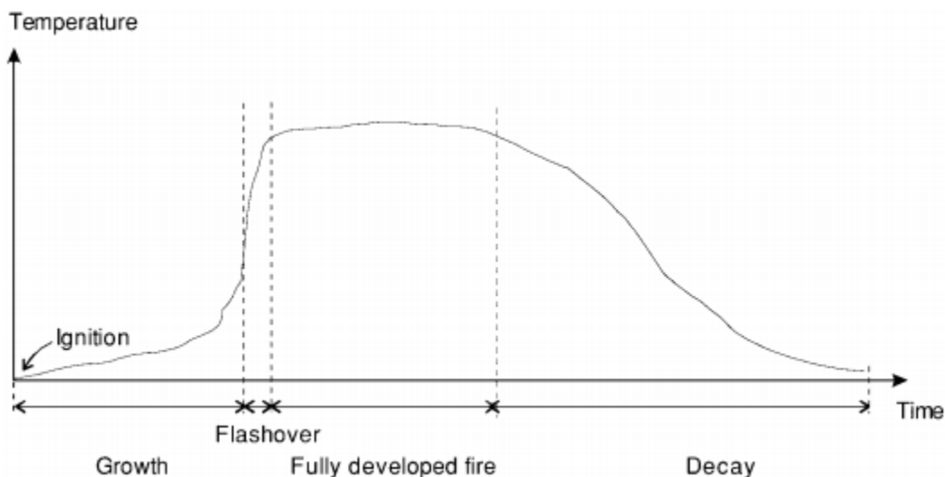
Figure 1 Fire development in enclosure in terms of temperature [10]
