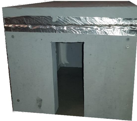
Figure 4 Test room, non-combustible material
