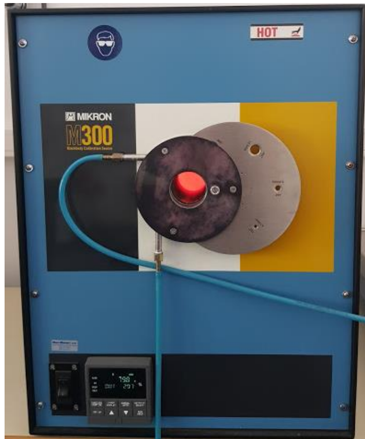
Figure 37 Oven used for determine response time
