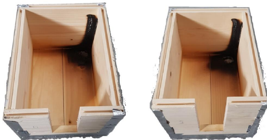
Figure 21 Exp 11 (left) & Exp 12 (right) after first ignition of ceiling
