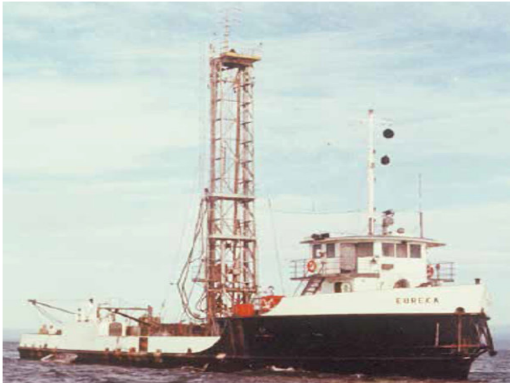
Figure 1 The Eureka was the world's first automatically positioned vessel. Picture courtesy of Howard Shatto.
