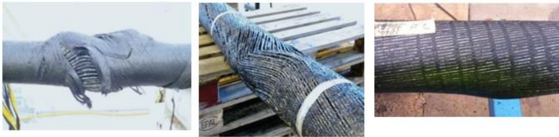
Figure 17 Images from left to right: 1. Bird-caging, 2. Lateral buckling, 3. Radial buckling (Tyrberg, 2015)
